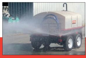
Rear spray bar is capable of producing a cone of water from 8' (gravity flow) to 36' (pressurized flow)
