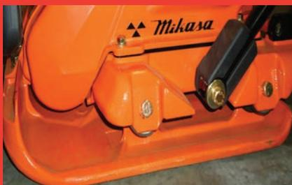
**Baseplate Design** - open for easy removal of rock build up and special contour for asphalt applications.
