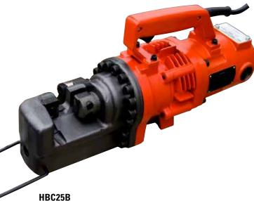
Maximum Cutting Diameter In (mm) 1 (25) #8 rebar grade 60 Voltage/Amperage 115V 60Hz 13 amps Maximum Cutting Speed 3.5 sec.
