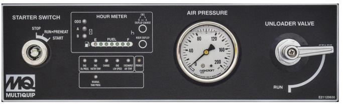
Control Panel monitors compressor and engine statistics:
