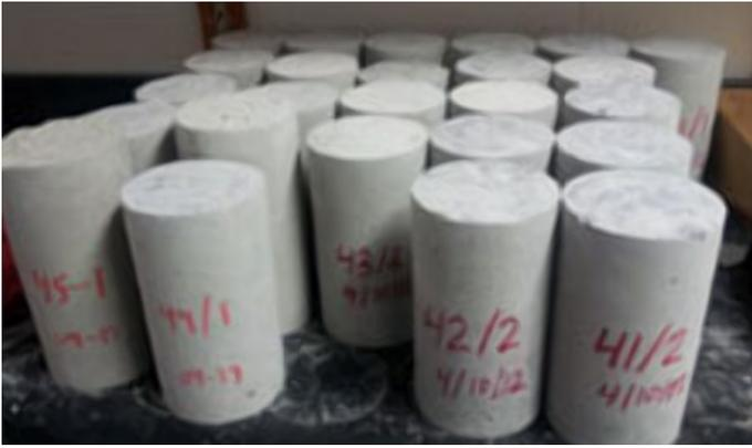
are filled with concrete during the operation of placement as specified by ASTM C172, “Standard Method of Sampling Fresh Concrete”, and ASTM C31 “Standard Method for Making and Curing Concrete Test Specimens in The Field”. The cylinders are moist-cured at about 70 degree F, generally for 28 days, and then tested in the laboratory at a specified rate of loading. The compressive strength obtained from such tests is known as the cylinder strength  $f_c'$  and this term is used in design purposes.
